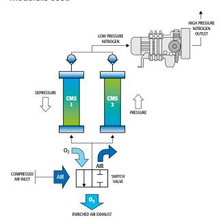
Claind has improved the PSA technology with the exclusive internationally patented FAST PURITY<sup>TM</sup> system, which ensures:
